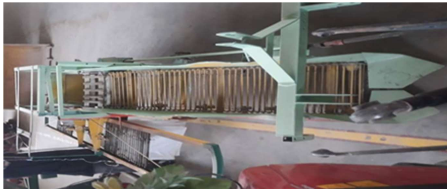
Figure (1) components of potato digger with side and rear conveyor.
