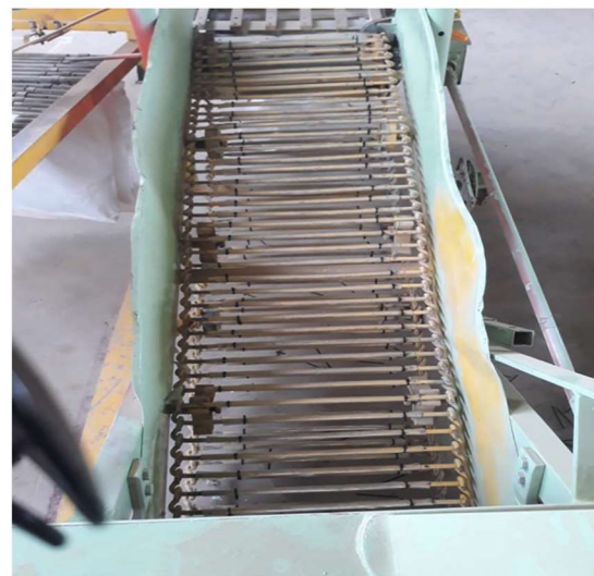
Figure (2) rubber coated Conveyor
