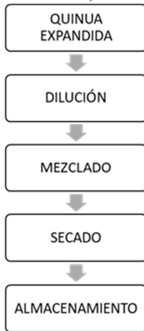
Figure 2. Diagram of the flavoring process of expanded quinoa snack. (orange and chocolate)
